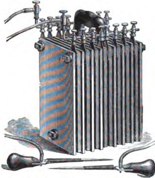
FIG. 20.—BATTERY AND ELECTRODES USED BY CUTTER.
